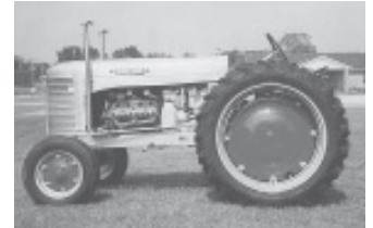
Richard Lyman restored this 1955 Silver King tractor, built in West Virginia, with a Ford flathead V-8 100 hp engine.
