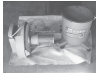
Lowell Blakely adapted an old air filter from his skid loader to fit his Sears shop vac.
